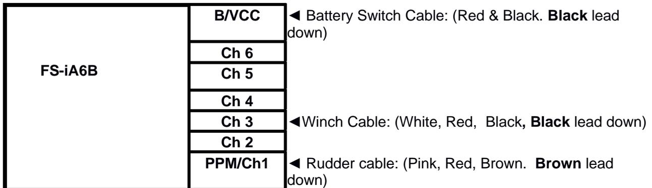
Note that labels shown on Rx do not exactly align with ports below.
